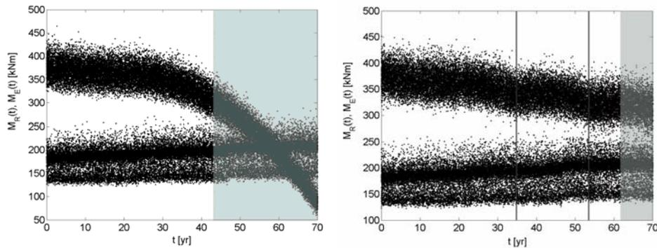
Fig. 2 The time dependency of the resistance and the load effect: (a) member without secondary protection, (b) member with two secondary protective paintings
