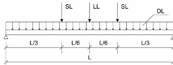
Fig. 1 Scheme of a simply supported reinforced concrete beam
