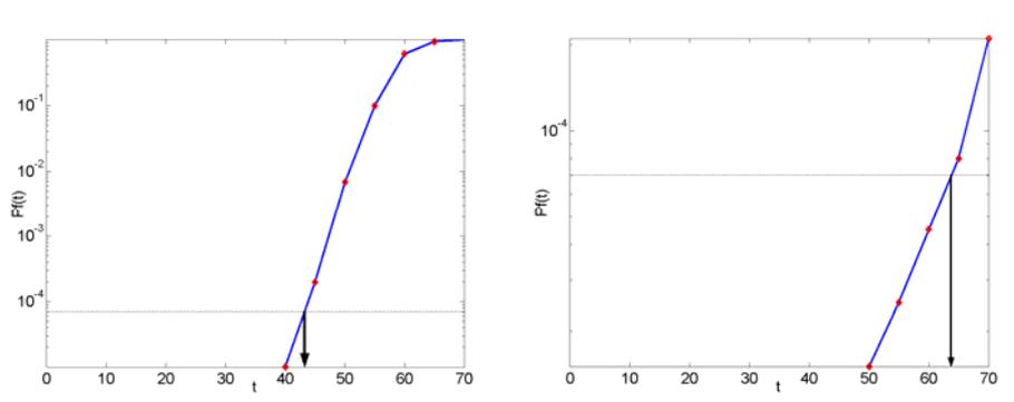
Fig. 3 The curves of probability of failure: (a) member without secondary protection, (b) member with the two secondary protective paintings
