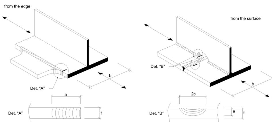
Fig. 1: Characteristic propagation of cracks: (a) from the edge, (b) from the surface
