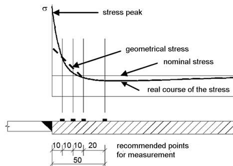
Fig. 3: Installation of sensors and courses of stress
