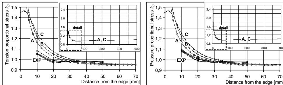
Fig. 6: Comparison of measured stress (selection) and FEM stress
