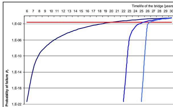
Fig. 7: Dependence of the failure probability  $P_f$  on operation years of the bridge and determination of inspection intervals for the designed failure probability  $P_d=2,277.10^{-2}$ .
