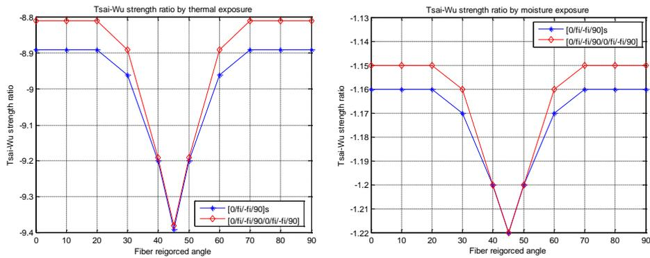
Fig. 2. Thermal and moisture strength of ratio versus fiber reinforced angle
