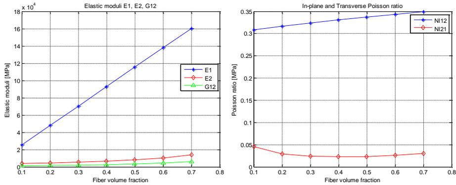
Fig. 1. Elastic properties versus fiber volume fraction.
